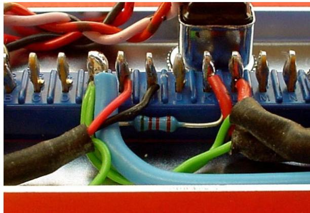
► In situations where the **fader connection is not used** (most Neve 45 series consoles except the original BCM10's) then the resistor remains in place.
