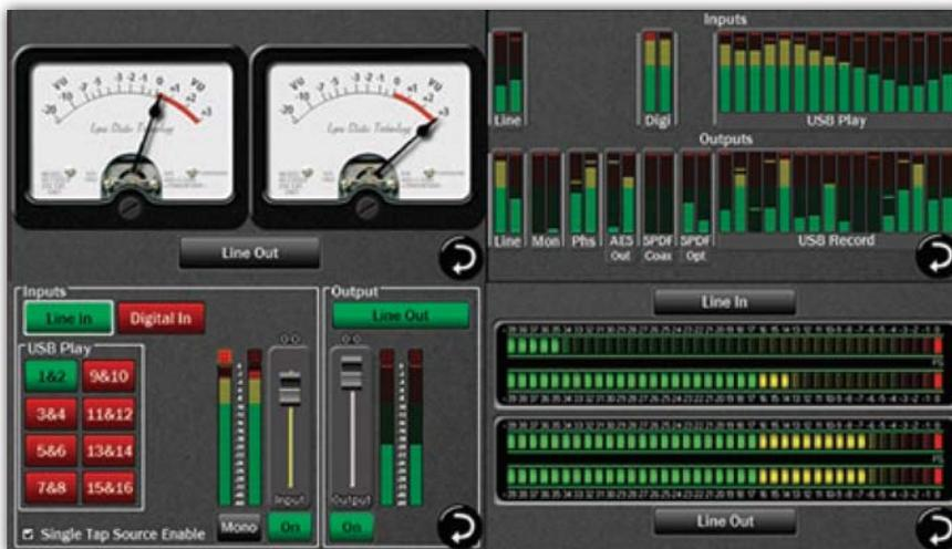
» The heart of the Hilo is the routing and mixing facility, configured by selecting the desired output pair in the Routing sub-menu. The display shows the output on the right, with a stereo meter, on-off button and digital level fader, and the available input sources on the left, again with another meter, fader, and a mono button. Active inputs are coloured green, while inactive or muted ones are red and the selected input is highlighted with white box edging.
