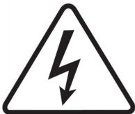
The lightning bolt with arrowhead symbol within an equilateral triangle is intended to alert the user to the presence of uninsulated “dangerous voltage” within the product’s enclosure that may be of sufficient magnitude to constitute a risk of electric shock to persons.
