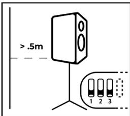
The speaker is on a monitor stand, at least .5 meters (about 20 inches) away from any walls. **This is the ideal position for the loudspeaker.**
