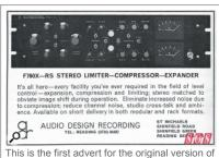
the F760X RS stereo limiter-compressorexpander (published in Studio Sound magazine in April 1973), showing the original front-panel layout. A revised version with the more familiar control arrangement, and called the Compex for the first time, was first shown in 1975.
