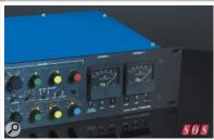
The gain-reduction metering includes a stereo coupling mode, and is quite sophisticated — it's best used in conjunction with the indicator lights, which hint at which processes are triggering the gain reduction!
