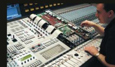
Extensive test and line up procedures. (Note: Ribbon extenders used for test purposes only)
