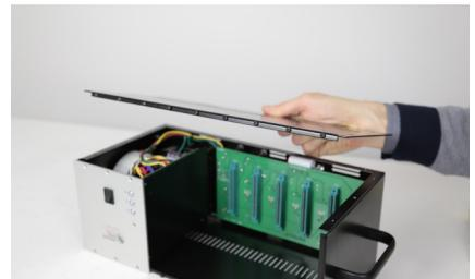
Using your #1 Phillips-head, remove all ten (10) screws from the bottom panel and the three (3) front panel screws at the bottom of the rack. Remove the bottom panel and set it aside.
