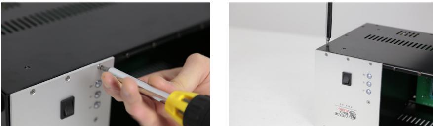
Put the bottom panel back in place, replace the bottom three (3) front panel screws, and then all ten (10) bottom panel screws with your #1 Phillips-head.
