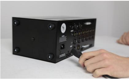
Turn off the rack, unplug the power cable, remove all audio connections and any modules you may have installed.
