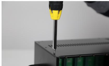
Put the top panel back in place, replace the top three (3) front panel screws, and then all ten (10) top panel screws with your #1 Phillips-head.
