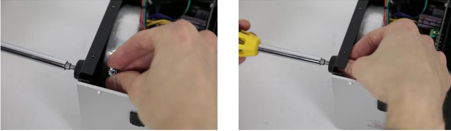
Carefully install the bottom two (2) bottom feet in the side of the rack through the existing screw holes. Secure the screws with your #2 Phillips-head and the hex nuts provided separately with your rack.
