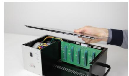
Using a #1 Phillips-head, remove all ten (10) screws from the bottom panel and the three (3) front panel screws at the bottom of the rack. Remove the bottom panel and set it aside.
