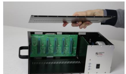
Using a #1 Phillips-head, remove all ten (10) screws from the top panel and the three (3) front panel screws at the top of the rack. Remove the top panel and set it aside.
