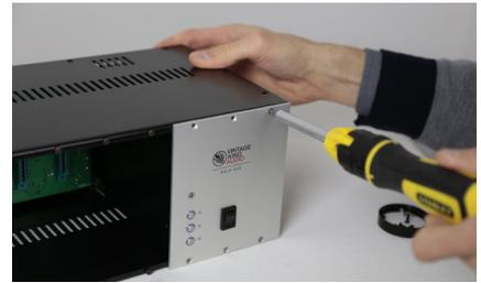
Put the top panel back on with the ten (10) top screws, then do the same with the bottom panel and ten (10) bottom screws. Then reinstall the six (6) front panel screws.
