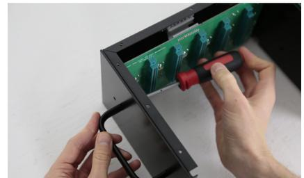
Put the left rack ear (with VK logo) in place and reattach the handle, securing the screws through the rack ear. Tighten screws to secure the rack ear with your #2 Phillips-head.
