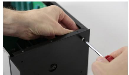
Put the right rack ear in place and use the hardware supplied with the rack ear kit. Insert the screws with washers through the outside of the rack and tighten the supplied hex nuts on the inside using your #1 Phillips-head.
