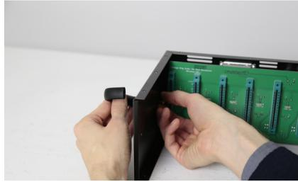
Using a #2 Phillips-head, remove the two (2) screws securing the handle. Set the screws and handle aside; they will be used to secure the left rack ear in the next step.
