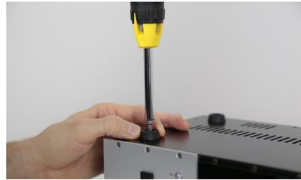
Using a #2 Phillips-head, unscrew all four (4) rubber feet from the bottom of your rack. Keep them together in a plastic bag, in case you ever want to put them back on.
